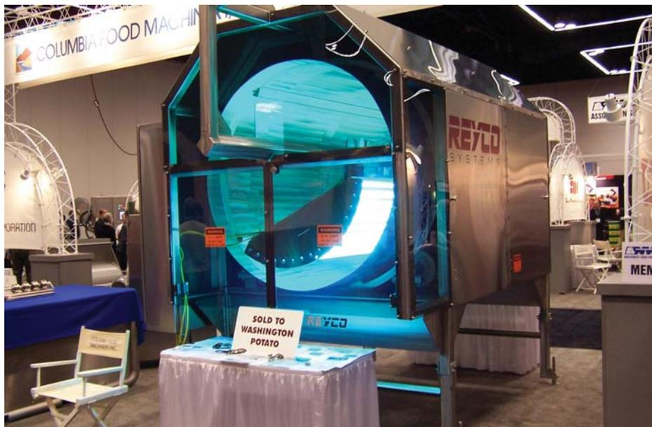
An array of short-wave UV lamps provides a kill step against mold, viruses and bacteria in this tumbling drum bound for duty in a potato processing plant. Source: Steril-Aire Inc.
